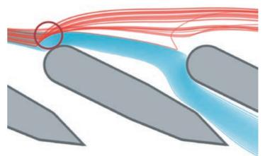
Figure 1: Ricochet effect visualization from (Divi et al., 2018). The blue and red lines show pathlines of water and particles contained in the flow. The grey geometry shows the filter elements.
