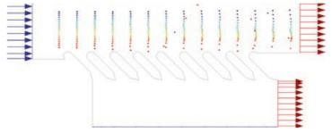
Figure 7: Particle location visualization for an inlet flow velocity of 2 m/s.
