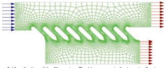
Figure 3: Visualization of the filter setup. The blue arrows indicate water flowing into the filter inlet. The red arrows indicate water flowing out of the two outlets. The top and bottom outlets are the dirty and clean outlets respectively. The green lines represent the discrete 2-dimensional mesh generated for simulations.
