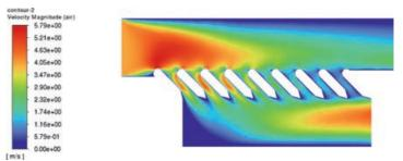
Figure 5: Flow velocity profile for an inlet flow velocity of 4 m/s.
