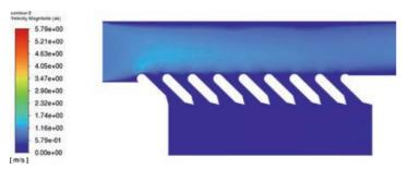
Figure 4: Flow velocity profile for an inlet flow velocity of 1 m/s.
