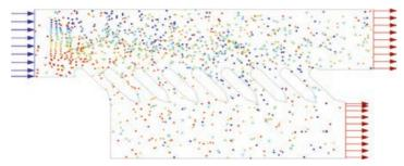
Figure 6: Particle location visualization for an inlet flow velocity of 0.25 m/s
